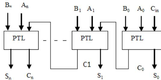
**Figure.2** Design of n-bit PASTA using Mux
